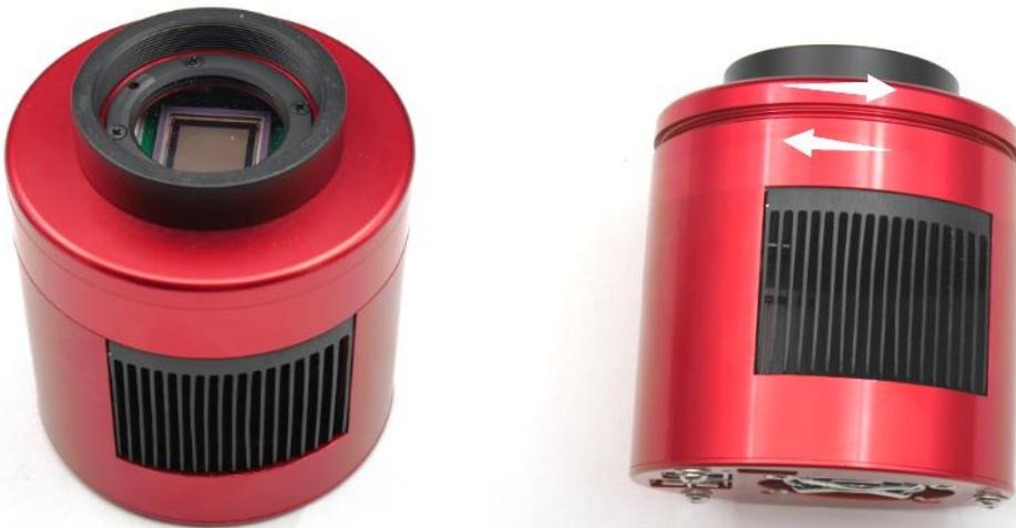
2. Uncooled camera is similar, anticlockwise screw the front piece hardly, and hold camera body by another hand.
